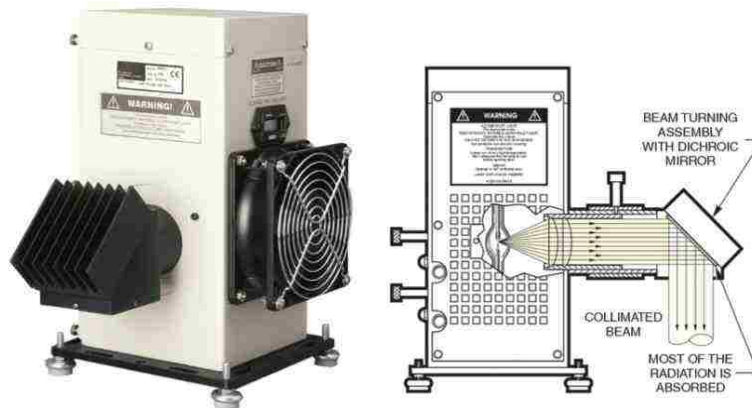
Figure 2.2: Newport Solar Simulator lamp output configuration showing the dichroic mirror that absorbs infrared wavelengths and reflects other light at a right angle (atmospheric attenuation filter, AAF, not shown). Images obtained from the manufacturer.
